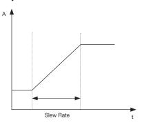
In CC mode, users can control the rate or slope of the change in current in a transient response test. Set the slew rate as slow as 0.0001 A/ $\mu$ s or as fast as 1 A/ $\mu$ s depending on the model and selected current range.
