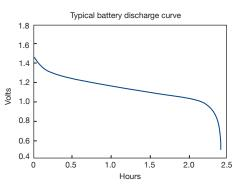
Built-in battery test function to calculate the Ah characteristic and capacity of a battery using a fixed current load discharge. Specify stop conditions for cut-off voltage, capacity level, and time up to 27 hours.
