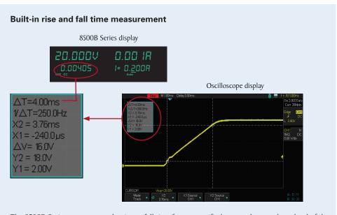
The 8500B Series can measure the rise or fall time from a specified start and stop voltage level of the measured input without the need for an oscilloscope. This function can also be used as an internal timer to count how long the input has been enabled.
